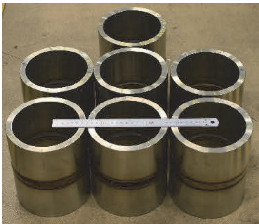
Fig. 5 Appearance of pipe butt-welded joint.
